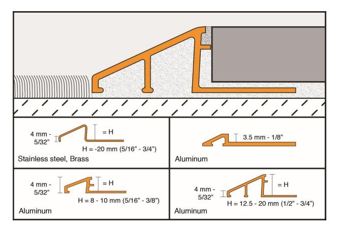
Recommended for all Liquid Elements self-levelers when transitioning to tile or other flooring systems of different height.
