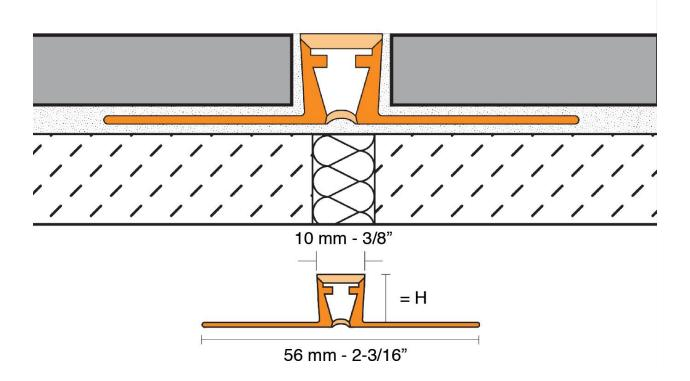
Recommended to use as an expansion joint with Liquid Elements Crush.
